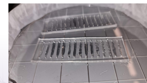
The PDMS film is lined with the capture antibody and allowed to incubate overnight.
